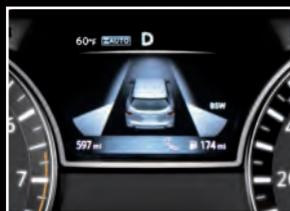
**Advanced Drive-Assist® Display.** From trip computer to 4WD torque distribution, the Advanced Drive-Assist® Display serves up info right in front of you – helping to minimize time looking away. Its intuitive 3-D depth and tilt design help you take it all in quicker.<sup>5,6</sup>
