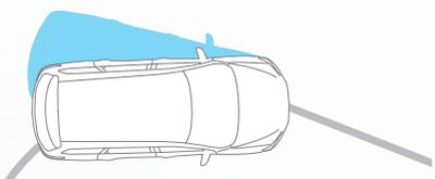
**Vehicle Dynamic Control (VDC).** Also known as stability control, VDC monitors your steering path and braking to help you maintain your steered path under certain conditions by reducing engine output and/or applying brake pressure to specific wheels.<sup>7</sup>
