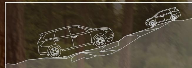
**Ups and Downs.** When your travels take you on steeper paths, hill start assist helps prevent rollback when starting and driving away on an incline. Hill descent control<sup>6</sup> helps make going down steep grades more manageable by automatically adjusting your speed and brake pressure to help keep you going at a controlled speed.
