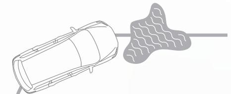
**Traction Control System (TCS).** When TCS senses drive-wheel spin, it responds by reducing throttle or applying brake pressure to help maintain traction.<sup>7</sup>
