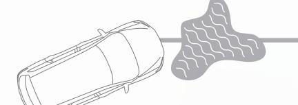
**Traction Control System (TCS).** When TCS senses drive-wheel spin, it responds by reducing throttle or applying brake pressure to help maintain traction.
