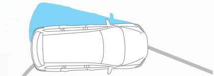
**Vehicle Dynamic Control (VDC).** Also known as stability control, VDC monitors your steering and braking to help you maintain your steered path under certain conditions by reducing engine output and/or applying brake pressure to specific wheels.<sup>7</sup>
