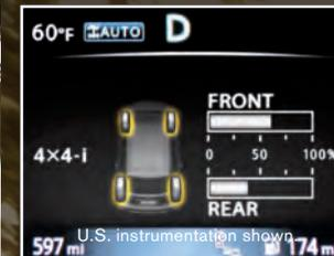
**Balance of Power.** The Advanced Drive-Assist Display illustrates the Pathfinder dividing the power between the front and rear axles, helping to give you the available traction and control you need.<sup>4,5</sup>
